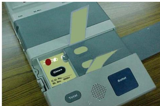
ECIL Machine Sealing the with inner door with Special Tag
